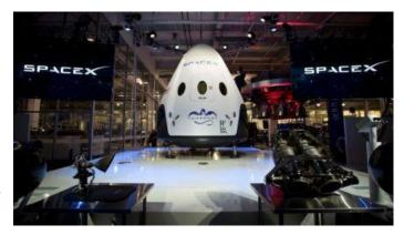
The Super Draco engines have 16,000 pounds of thrust. That is 160 times more powerful than the Draco manuvering rockets. There are 8 Super Draco rockets on the new crewed spacecraft. If 2 fail, no problem they can still land on land safely with 6 motors working. They can also restart and also be throttled.
